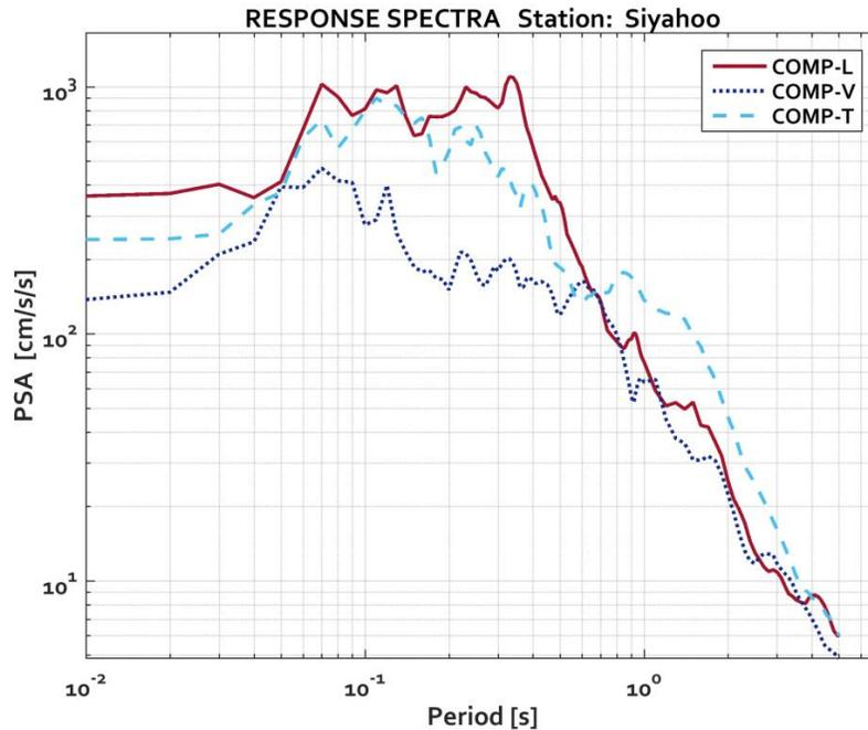
Figure 4. Recorded acceleration time histories (top) and acceleration response spectra of first earthquake at about 19 km epicentral distance.
